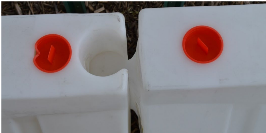
The temporary barriers (less than 40 pounds dry) lock together and have capped fill-holes for adding water, water and antifreeze, or sand. They also have drain plugs on the bottom if they will be emptied and stored for the winter.
